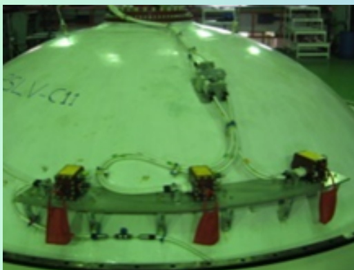
Fig. 3. Dual safe arm based ignition pyro-circuit
